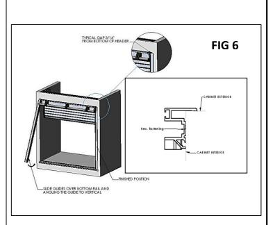
At this point the door should move freely up and down thru the guides onto the roller. It may be necessary to make some adjustments to the counter balance to assure proper tension. (Please see instructions for adjusting counter balance tension if this is needed.)
