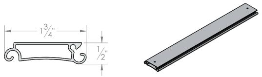
FOR ADDED RIGIDITY OUR 2EB SEALED SLAT CAN BE USED IN PLACE OF THE 2EA SLAT. IT OFFERS A DOUBLE WALL EXTRUSION ALONG WITH SEALS TO PROTECT FROM THE ELEMENTS
