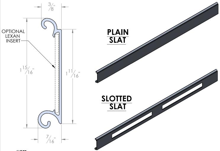
THE 2 EA SLAT OFFERS A SOLID OR SEE THROUGH PROFILE. (DIMENSIONS ABOVE). WE ALSO OFFER LEXAN INSERTS FOR OUR SLOTTING SYSTEMS, OFFERING A SEE THROUGH FORMAT WITH ADDED SECURITY OR COULD BE LEFT OUT FOR A VENTILATION OPTION. THE SLOTS CAN BE ARRANGED IN ANY ARRAY TO FIT OUR CUSTOMER'S NEEDS. AVAILABLE IN ANODIZED OR POWDER COATED FINISHES.
